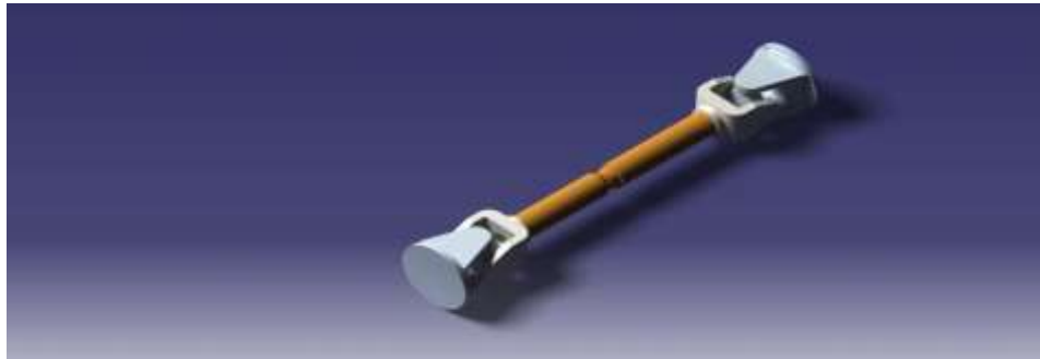
Fig 6. CATIA Model of Propeller Shaft
